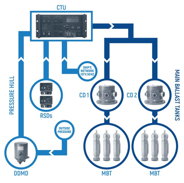
The Control and Test Unit (CTU) as well as the Remote Starting Devices (RSDs) and the Diving Depth Measuring Device (DDMD) are located in the pressure hull of the submarine whereas the Cable Distrubutors (CD) and the Gas Generators are located in the main ballast tank (MBT).
