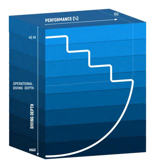
The RESUS system empties the forward MBTs in a very short time. Each generator produces gas at a nearly constant rate for about 13 seconds. Automatic step-by-step actuation of individual gas generators prevents overloading of the MBTs during the start phase. System performance has been successfully tested on board of different submarines.
