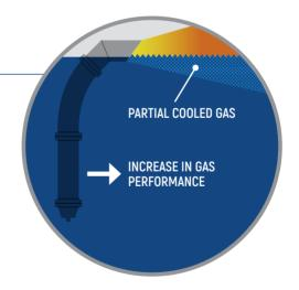
A steady gas bubble at the top of the main ballast tank allows the maximum gas performance de-ballasting the maximum water volume.
