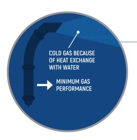
The hot gas provided by the RESUS system interferes with the cold water in the main ballast tank. The provided performance is reduced by thermic effects.
